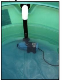
This is a high quality efficient magnetic drive submersible pump.
